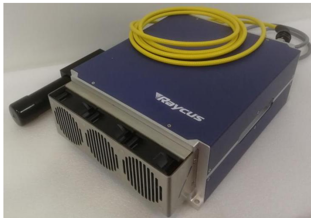
Figure 2. Photos of Raycus P20MX Pulsed Fiber Laser
