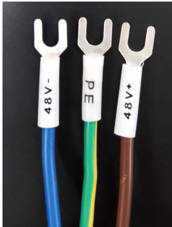
Figure 3 Definition of power line wires
