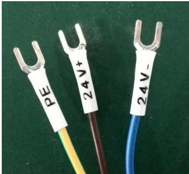
Figure 4 Definition of power line wires
