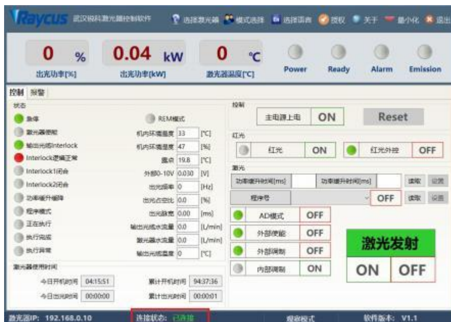
Figure 10 The main interface is displayed when the communication connection is normal
