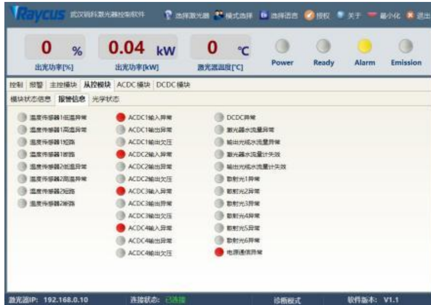
Figure 20 Slave control module alarm information interface
