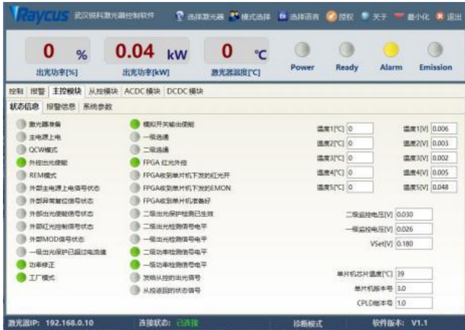
Figure 16 Main control module status information interface
