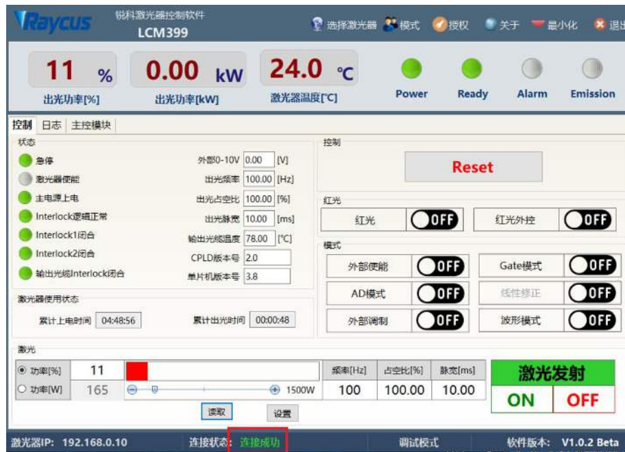
Figure 10 The main interface is displayed when the communication connection is normal
