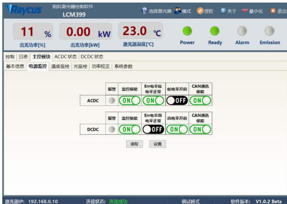
Figure 17 Alarm information interface of main control module
