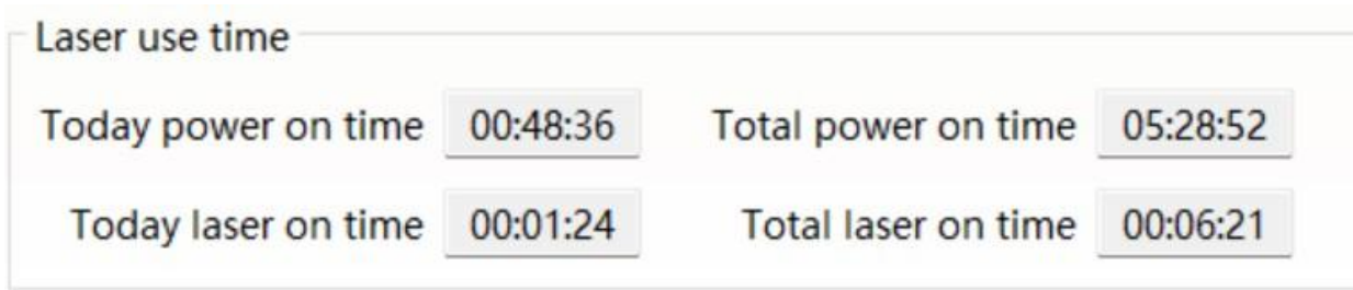
Figure 42 Display menu for accumulated working time of laser
