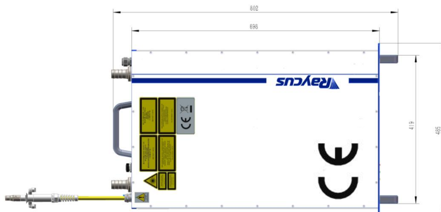
Figure 2b) Top and Side view (unit: mm)
