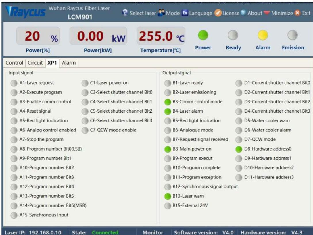
Figure 49 Interface Status Indication menu in Diagnostic Mode
