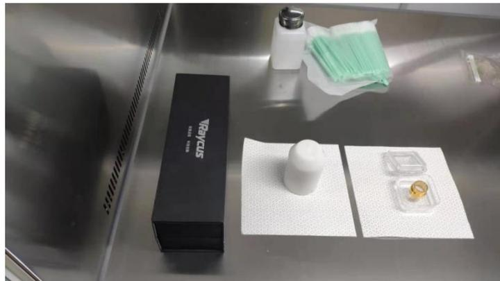
Figure 20 Accessories that customers need to keep: black protective box, white dust cover, type A end cover
