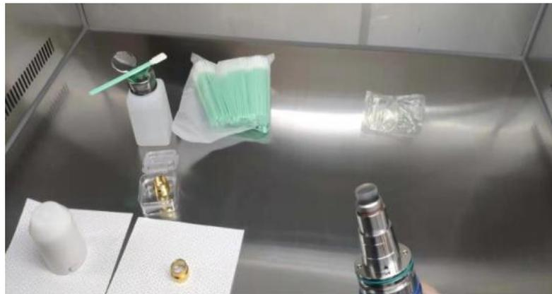
Figure 19: Removing the A-type end cap from the optical cable
