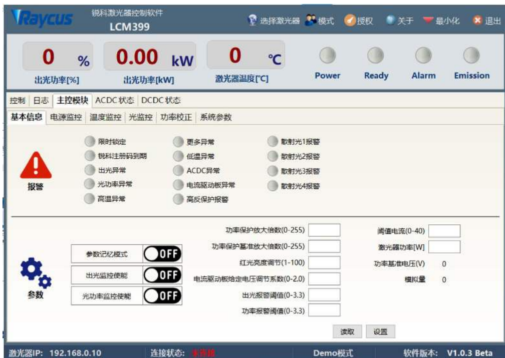
Figure 16 Main control module status information interface
