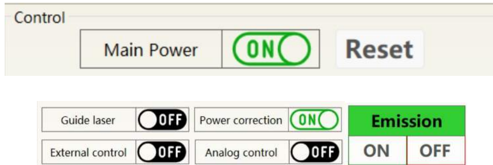
Figure 33 Display area for laser power on, mode selection, and light output control
