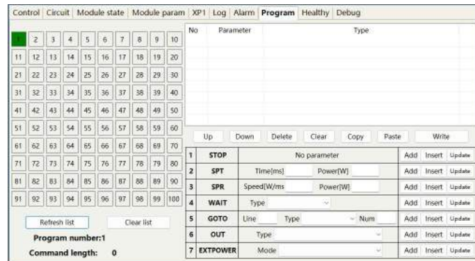
Figure 46 Operation menu for viewing the number of waveform stored inside the current laser
