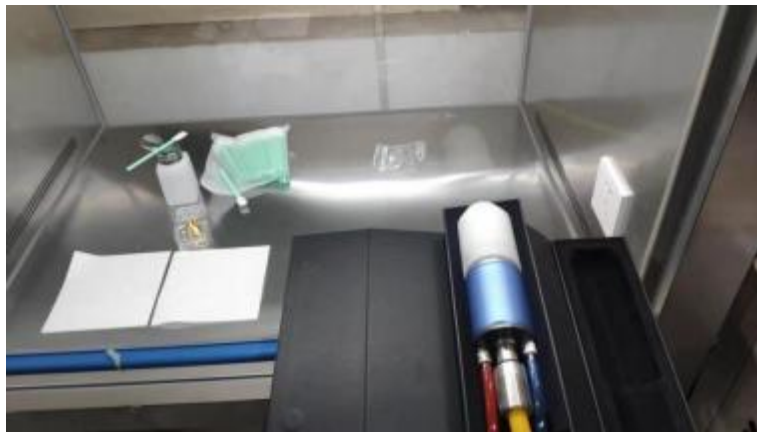
Figure 6 Output cable placed in the box
