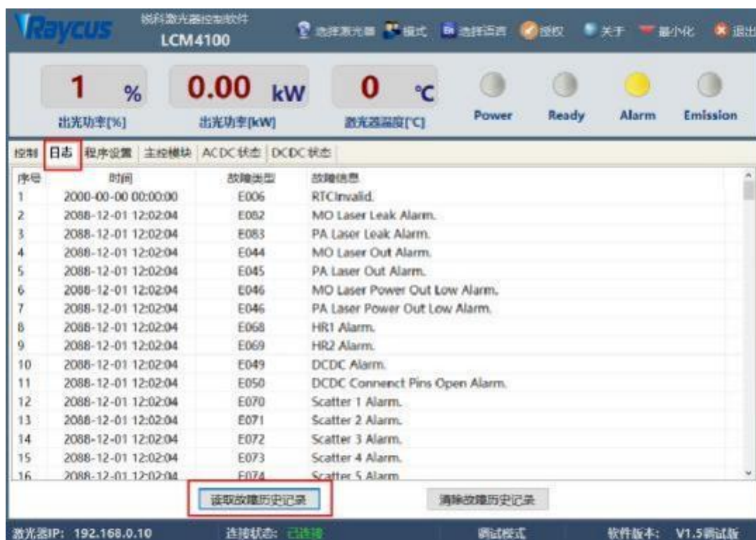
Figure 12 The alarm interface
