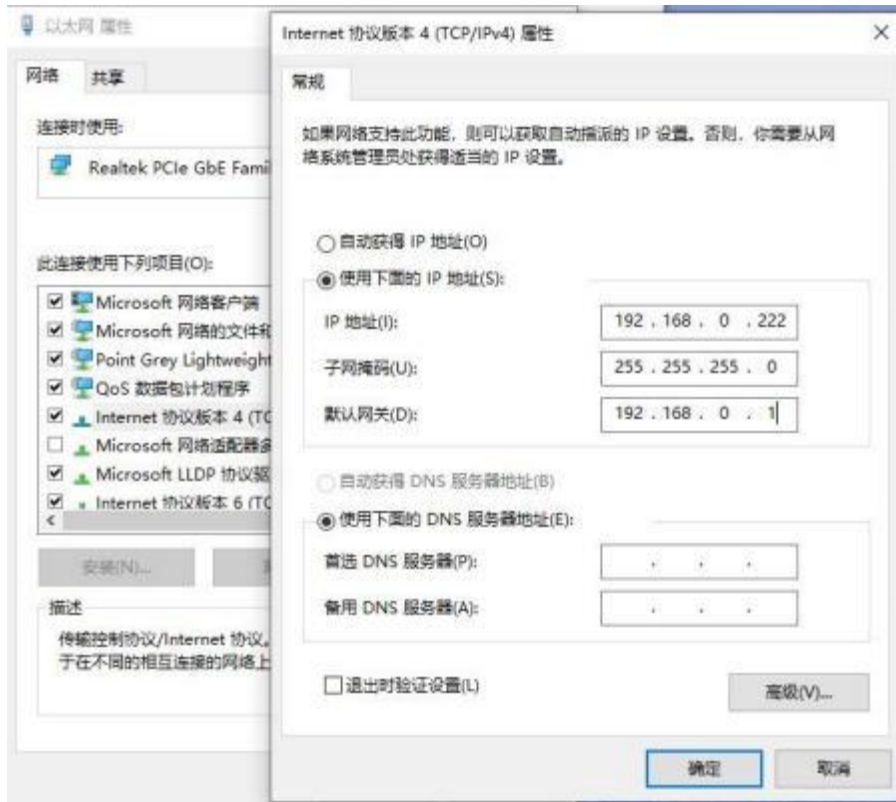
Figure 9 Steps of Ethernet Connection
