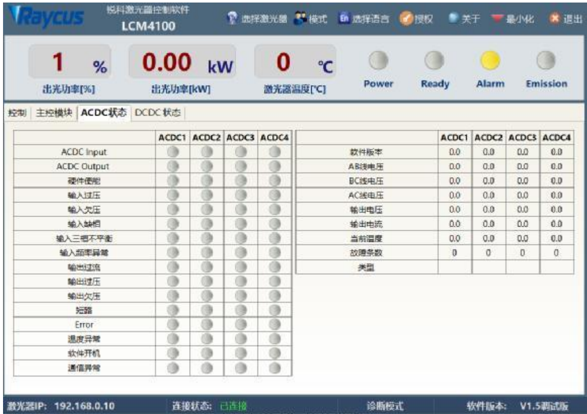
Figure 19 Slave control module status information interface
