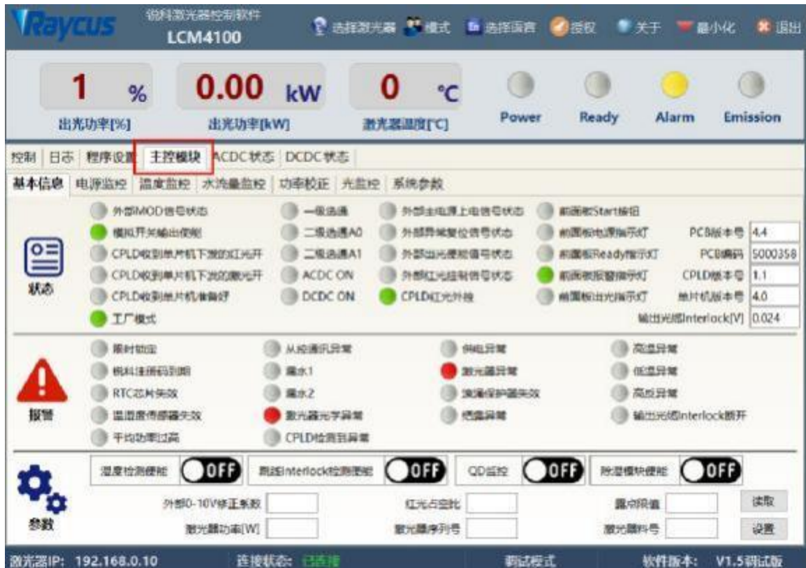
Figure 16 Main control module status information interface
