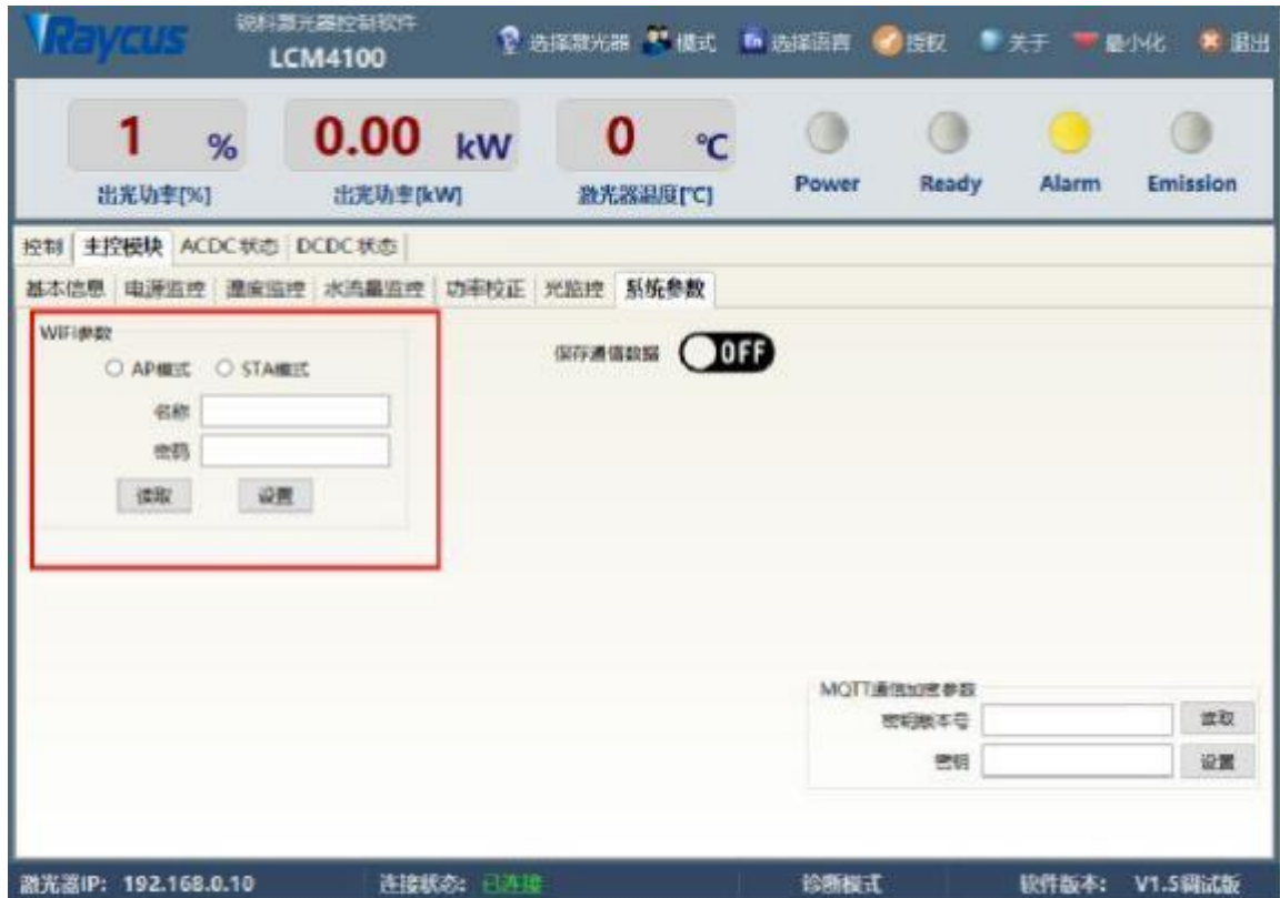
Figure 18 Main control module system parameter interface
